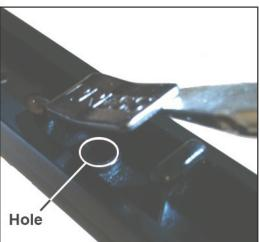
**2.)** Below the PRESS button is a hole to place the spring.
