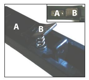
**4.)** Use screwdriver to hold down side A (as shown above,) then with pliers or another screwdriver push down side B.
