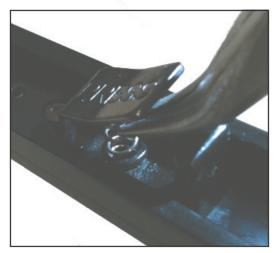
**3.)** With pliers, place the spring standing up into the hole and underneath the PRESS button.
